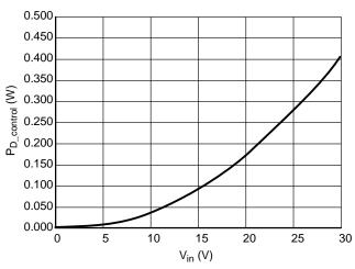
Figure 5. Power Dissipation vs. V<sub>in</sub> for the NUD4001
