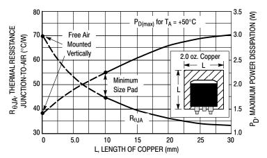
Figure 6. Thermal Resistance vs. Pad Size for a Typical D<sup>2</sup>PAK
