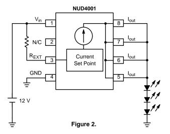
If the LEDs are 1 Watt devices (with a load current of 350 mA), the power dissipation in the NUD4001 is approximately 0.355 W. The detailed calculations are available in the NUD4001 data sheet.
