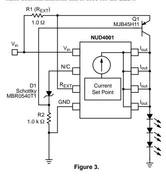
Looking at the Figures 1 and 2, for the NUD4001, one of the first things you will notice is that Pin 2 is marked as N/C (or no connect). Normally this is the case, but Pin 2 is also available to drive an external transistor.
